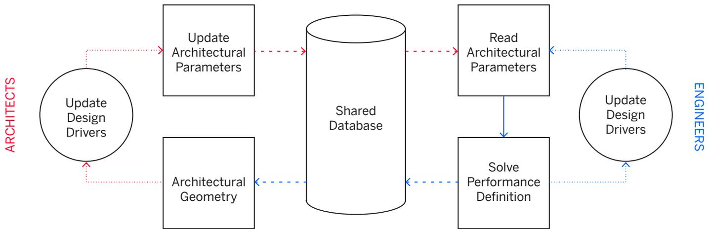
Figure 4. Analysis process is automated through the exchange of information takes place through a shared database
