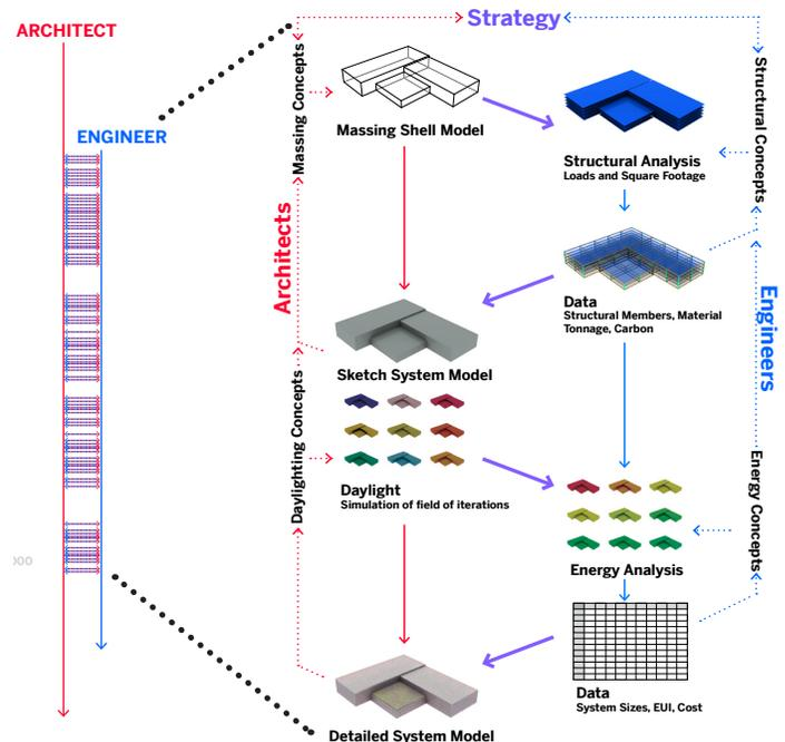
Figure 3. The design process continually builds on previous steps, retaining the ability to test new approaches from the beginning.
