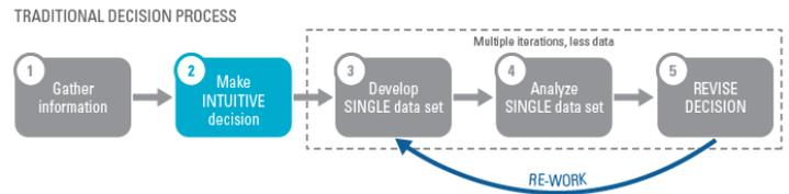
Figure 1: Linear decision making process during design
